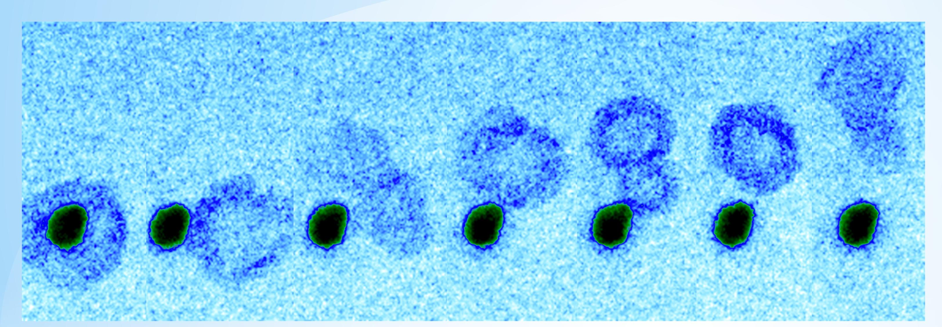
Water nanodroplet (dark blue) ~ 20 nm in diameter depins from a 10 nm gold nanoparticle (black) and continues on its way. A nanodroplet of this size contains about 1.4 million water molecules.
