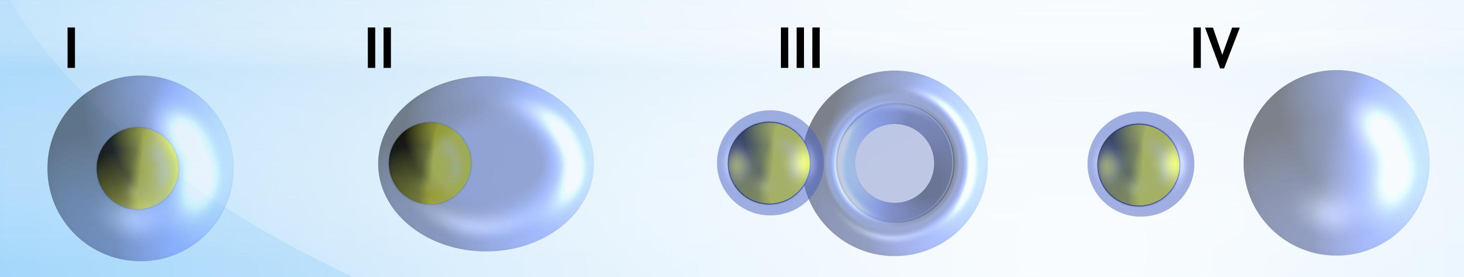
Schematic diagram of water nanodroplet depinning from nanoparticle.
